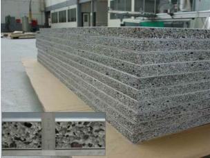
Fig. 4 Production of Aluminium Foam Sandwich at alm GmbH, Saarbrücken (Courtesy: H.-W. Seeliger).
