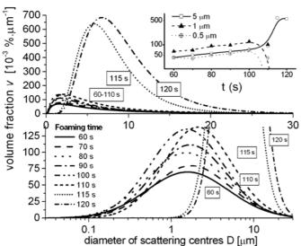
**Figure 2**. Pore size distributions v(D) in zinc foams. Upper: entire size range with inset showing volume fraction of scattering centres with 0.5, 1 and 5 µm size as a function of time, lower: semi-logarithmic representation restricted to scattering centres with small volume fractions.
