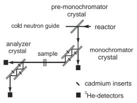
**Figure 1**. The experimental setup for USANS measurements.
