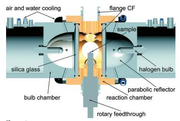
**Figure 1**Cross section of the radiation furnace.
