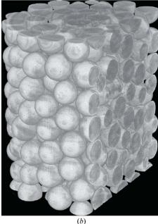
**Figure 4**Top: scanning electron microscope image of spherical monocrystalline copper particles marked with small holes by focused ion beam. Bottom: tomogram of these particles in an early stage of sintering (Grupp, 2008).
